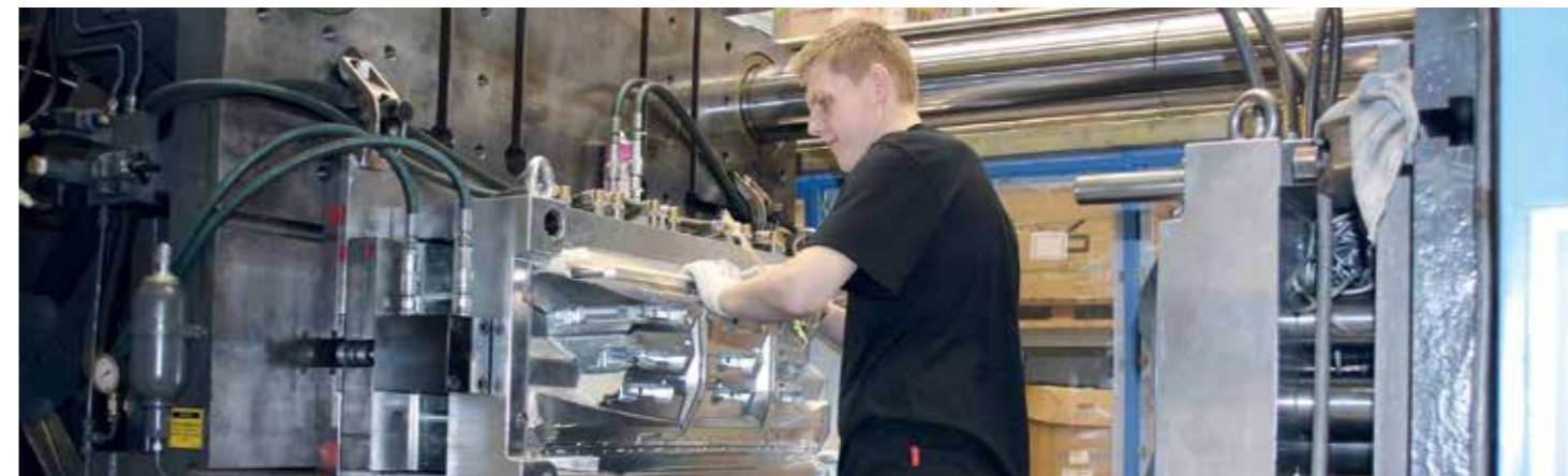
Flexibility is in demand: on average 5 mold changes per week and shot weights between 10 g and 2.8 kg.
