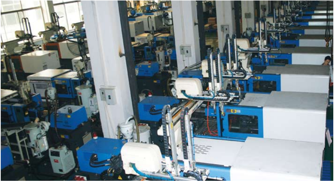
Altogether there are over 40 high equipped Haitian injection molding machines from 600 to 3,800 kN
