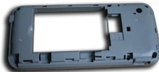
Top: Shell of a mobile phone, PCIABS, produced on a VE 1200/210h
