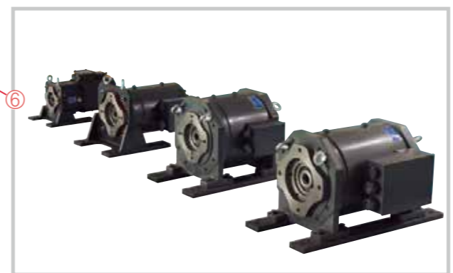
Figure ① Patented servo motor to gear pump design. The direct drive connection between the servo motor and the gear pump, provides excellent drive torque giving maximum acceleration and deceleration speeds for all machine functions. The patented drive system is a true advantage for high stability and repeatable molding conditions.
