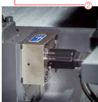
Figure ① Optimized platen design using FEA software. Higher rigidity and stability.
